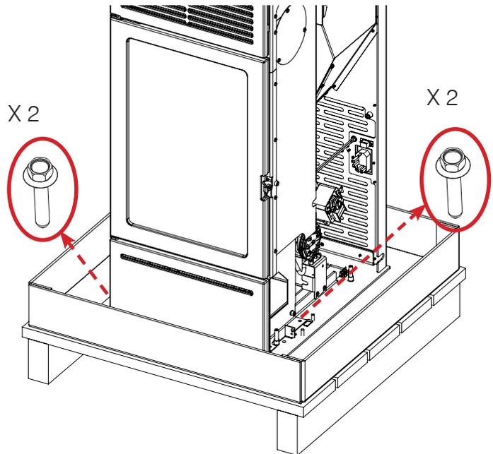
Fit the interlocking side panels and screw down the bolts on the back
