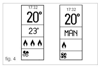
If timer programming is active, 3 and 4 are replaced by the day's timer programming with the current setpoint at the centre (figure 5) and the temperature displayed at the top right.
