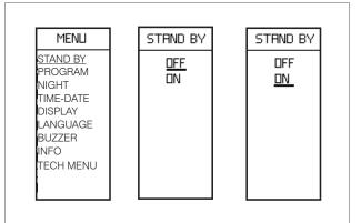
To access the function from the main menu (as indicated in the Menu section above), press the M button. Scroll using the +/- buttons and select the function by pressing OK.
