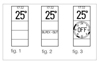
From the OFF page, press the ON/OFF button for 3 seconds to go to the ON page.
