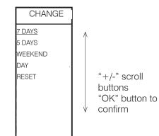
From the "CHANGE" function, in addition to changing/ viewing the "7 DAYS", "5 DAYS", "WEEKEND", "DAY" programming, you can **erase all time settings using the "RESET" function.**
