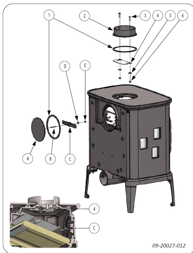
1. Remove the connection collar (2) and baffle plate (4) from the top of the appliance.
