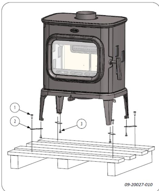
1. Remove the appliance from the pallet by removing the bolts (1).
