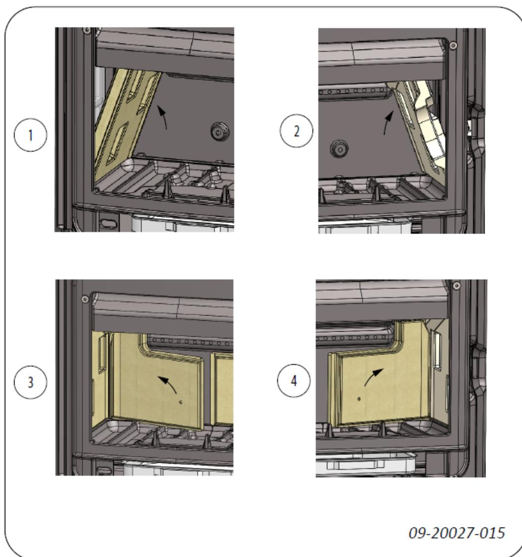
Order of inserting vermiculite inner plates:
