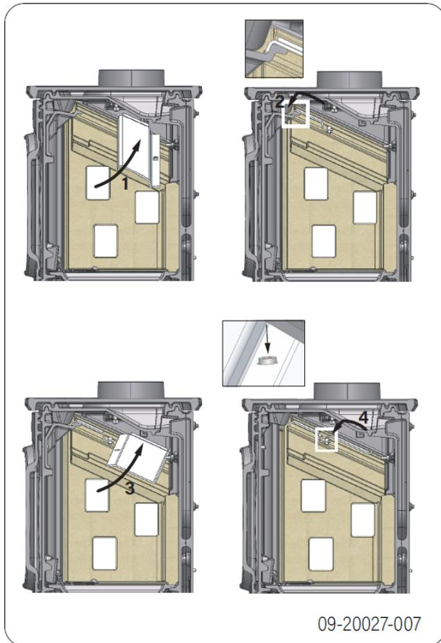
Order of inserting stainless steel baffle plates:
